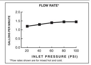
1.5 gpm/5.7 L/min. FLOW RATE
